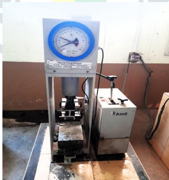
Fig.6: Experimental Setup of Flexural Strength Test
