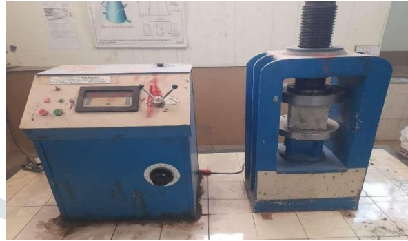
Fig.4: Experimental Setup of Compressive Strength Test
