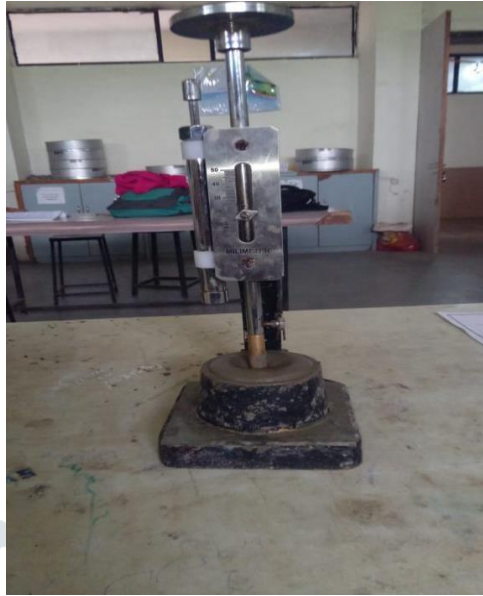
Figure No : 3.5 Vicat Apparatus
