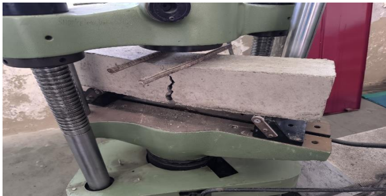
Figure No. 3.18 Flexural Strength On Beam
