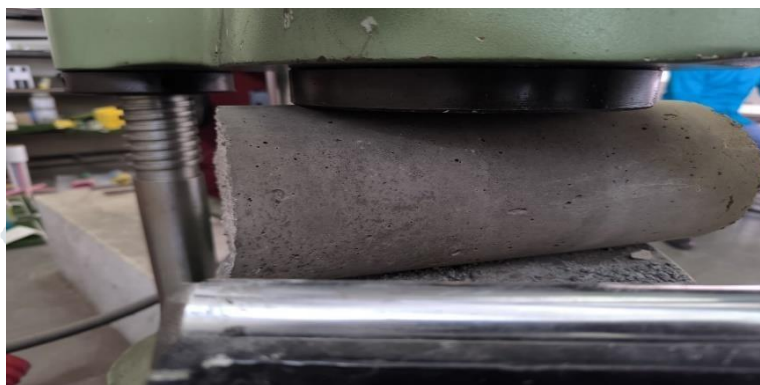
Figure No.3.19 Split Tensile Strength
