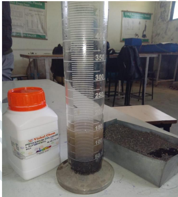
Figure No. 3.9 Silt Content
