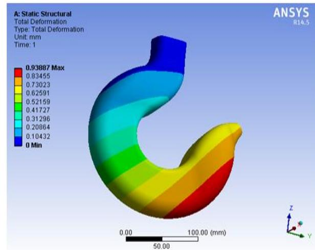
Fig.13. Deformation Plot for Rectangular CSA Of hook
