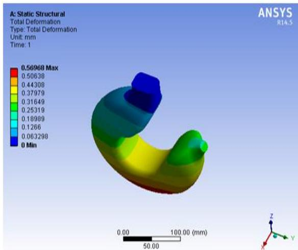
Fig.12. Deformation Plot for Trapezoidal CSA Of hook
