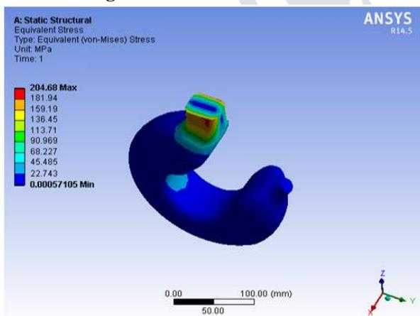
Fig. 10 Max. Equivalent (Von -Mises) Stress for Trapezoidal Hook
