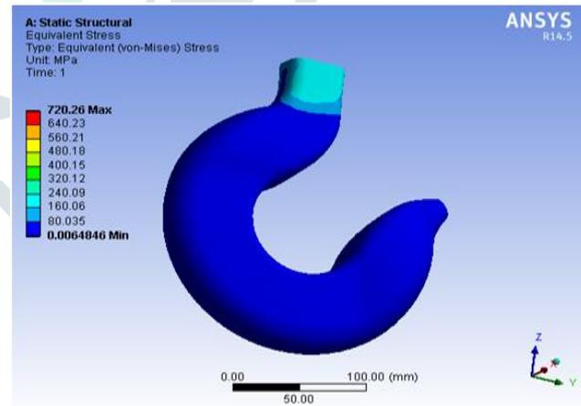
Fig. 11 Max. Equivalent (Von -Mises) Stress for Rectangular Hook
