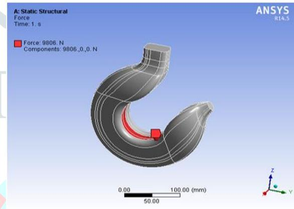
Fig.9 Boundary Conditions Applied On Rectangular Hook
