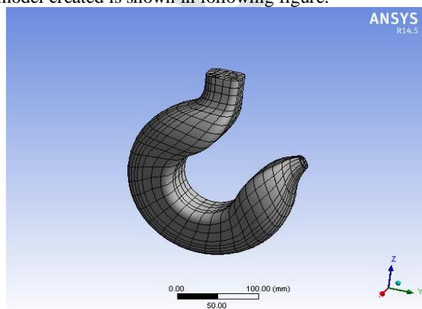
Fig.7. Meshing of Trapezoidal section
