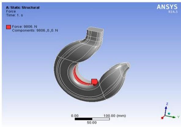
Fig.8. Boundary Conditions Applied On Trapezoidal Hook
