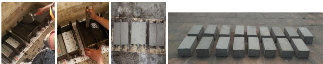
Figure. 2. Casting and curing of Geopolymer Bricks
